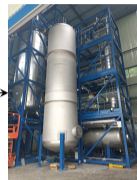
Distillation: remove radioactive impurities
