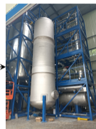
Distillation: remove radioactive impurities
