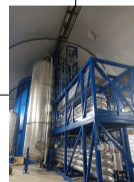
Gas stripping: remove Rn and O 2
