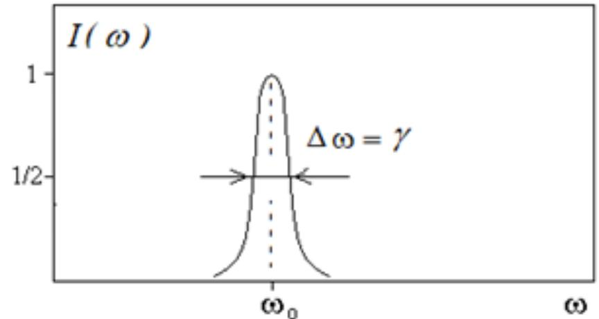
Decreasing in time the amplitude of oscillator  $x$  and the amplitude of the radiation field strength. Spectral width of radiation intensity  $I(\omega)$ .
