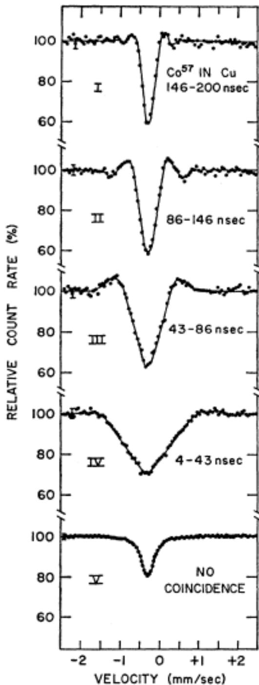
Delayed coincidence Mossbauer spectra using a source of  $^{57}\text{Co}$  in Cu-metal and an absorber of potassium ferrocyanide [4].
