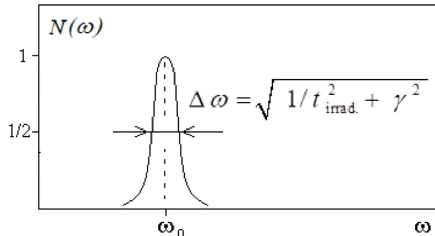
Spectral distribution of resonantly absorbed photons. Decay constant  $2 \gamma = \ln 2 / T_{1/2}$ ,
