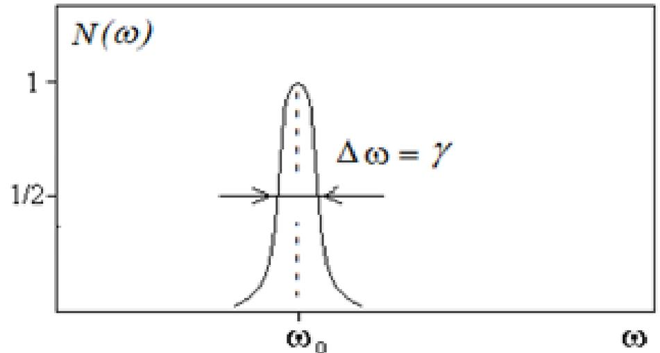
$$N(\omega) \propto \frac{1}{\left[ (\omega - \omega_0)^2 + \gamma^2 \right]}$$
