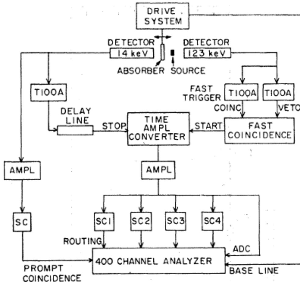
Schematic diagram of the fast-slow coincidence system used in the two-dimensional Mossbauer spectrometer [4]. The T100A units are fast discriminators, those designated AMPL are slow pulse amplifiers, and those designated SC are single channel pulse-height analyzers. Four 100-channel Mossbauer spectra can be determined simultaneously, corresponding to four delay time intervals.
