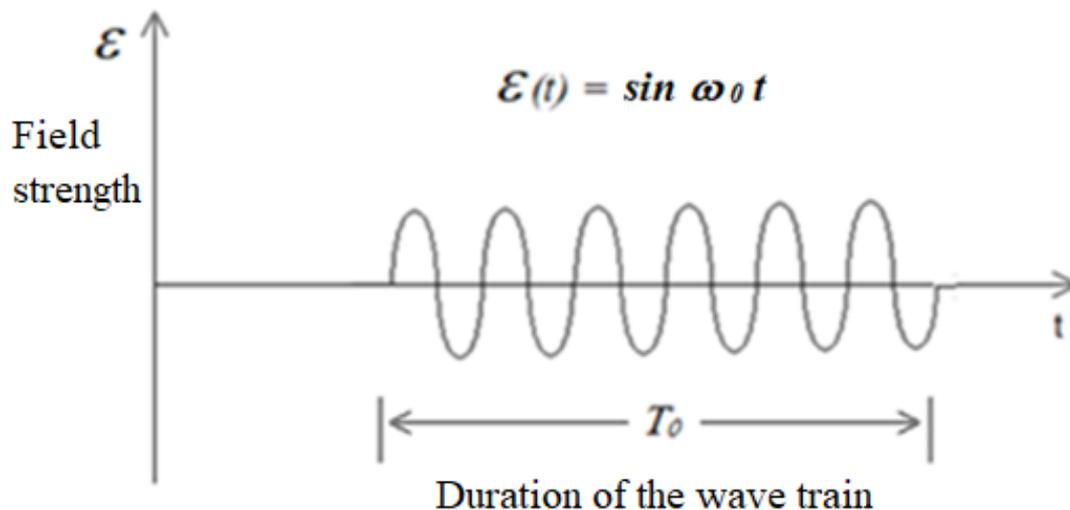
$$N(\omega) \propto \frac{1/T_0}{\left(1/T_0\right)^2 + (\omega_0 - \omega)^2}$$
