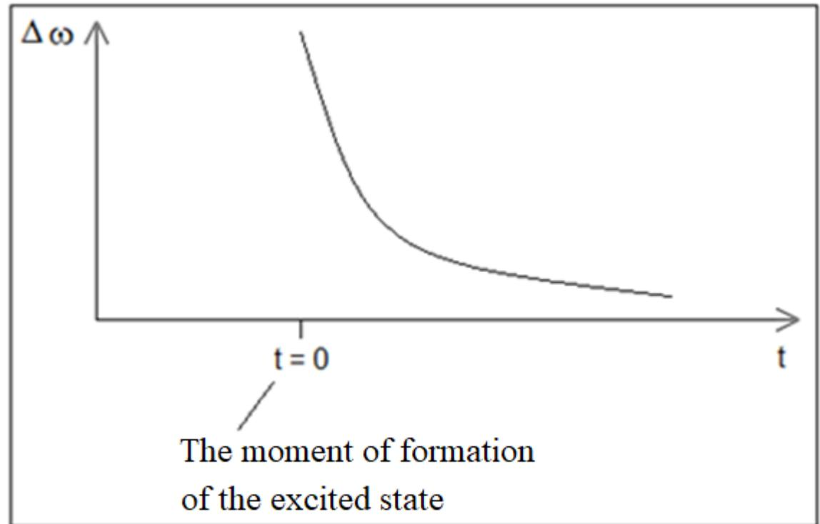
The spectral width of 14 keV photons decreases with age of the  $^{57\text{m}}\text{Fe}$  isomer.
