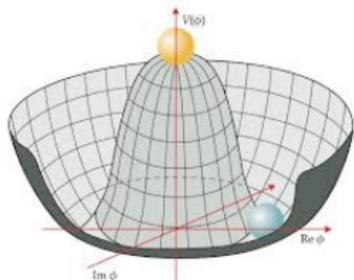
$$V^{\text{tree}}(v) = -\frac{a^2}{2}v^2 + \frac{\lambda}{4}v^4; \quad v_0 = \sqrt{\frac{a^2}{\lambda}}$$
