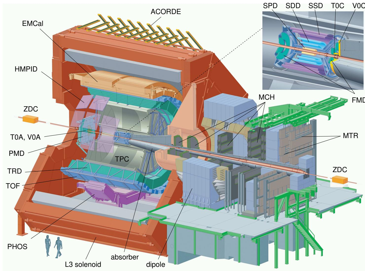
ITS, TPC and TOF are mainly used for reconstruction and identification of tracks
