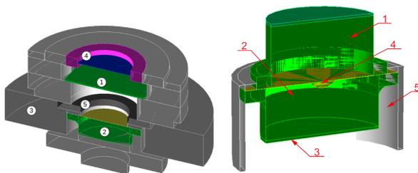
Left figure: target-detector spectrometer. Right figure: spectrometer with  $4\pi$  geometry.
