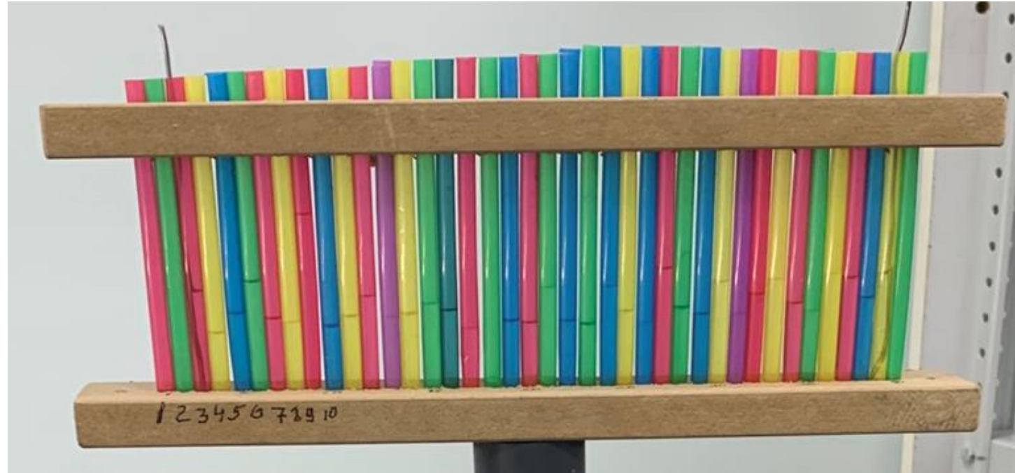
Phantom with tubes. There are I, Gd, La solutions and H 2 O in the tubes (Cocktail phantom)
