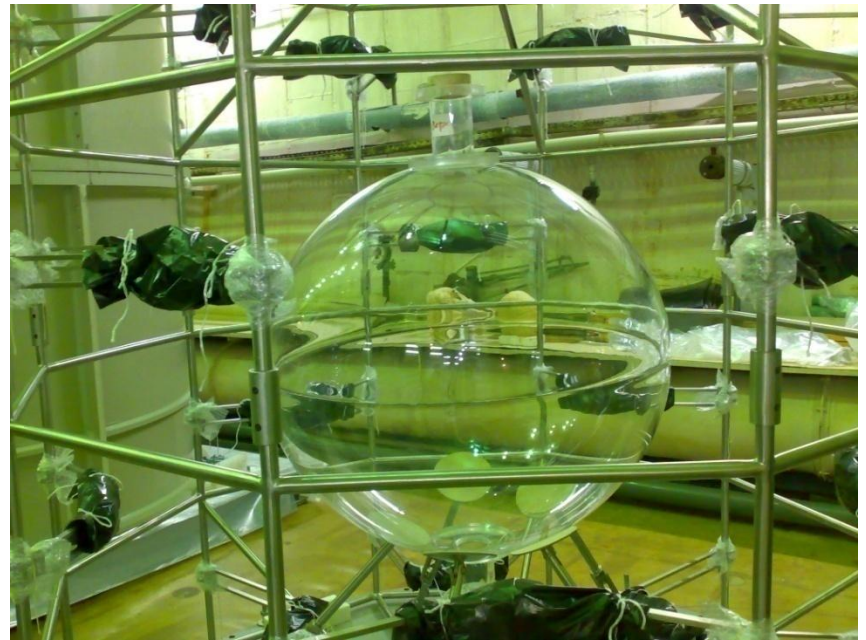
The acrylic sphere: inner diameter of 960 mm.
