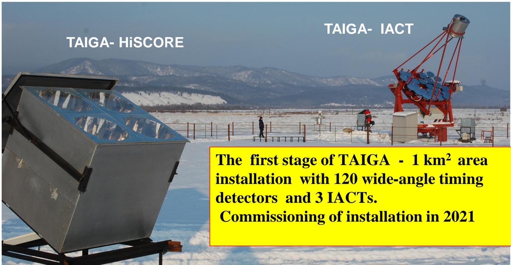
**The first stage of TAIGA - 1 km<sup>2</sup> area installation with 120 wide-angle timing detectors and 3 IACTs.**
