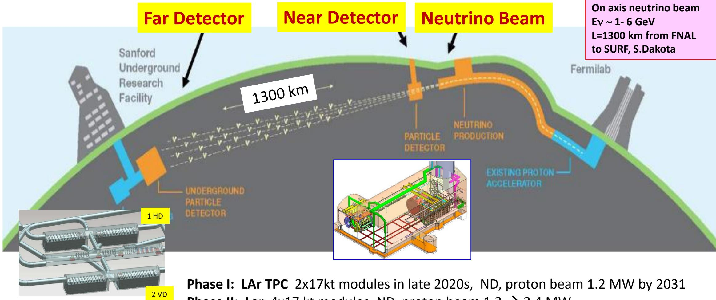
**Phase I:** LAr TPC 2x17kt modules in late 2020s, ND, proton beam 1.2 MW by 2031
