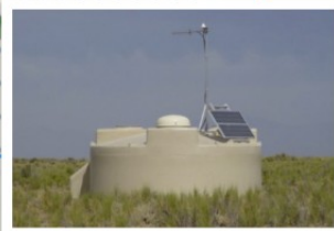
1665 surface detectors: water-Cherenkov tanks (grid of 1.5 km, 3000 km 2 )
