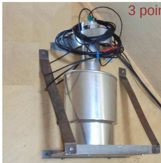
NaI crystal; 570 cm 2 installed in 3 points
