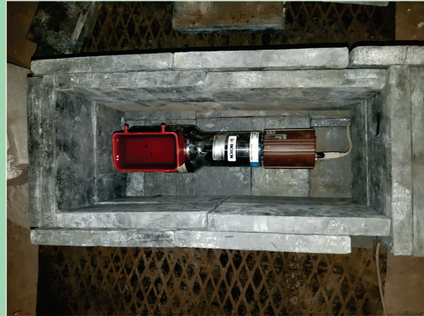
Figure 1. ORTEC firm gamma spectrometer (NaI(Tl), FWHM ~7.7% at 0.6 MeV, surrounded by 4-cm thick lead filters.
